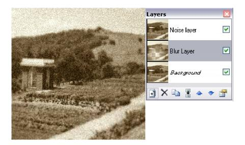
Open the Layer Properties window (f4.) Set the Noise layer blend mode to lighten.
